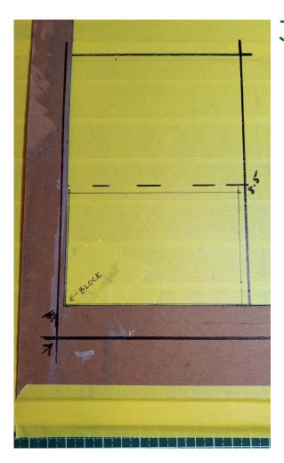
Using a steel ruler and Exacto knife, cut a 2nd piece of chipboard into an uppercase "L" and line up inner edge to your lino block mark. Tape down on bottom edge, transferring paper mark onto the "L" so you can see where to line up your paper. This "L" will hold the block in place while you print, and give you a definitive place to line up your paper (always register to bottom left corner, as shown).
